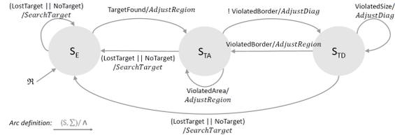
Figure 4. Mealy finite state machine diagram of the *ZoomController* logic.  $\mathcal{R}$  is a reset signal.
