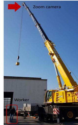
Figure 1. Crane load-view camera where red arrow points to, mounting on pendulum bracket.
